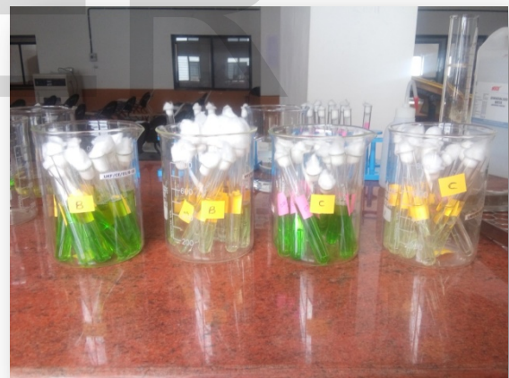
Fig.3. Test tubes filled with corresponding serial dilution samples in BGLB AND EC-Broth.
